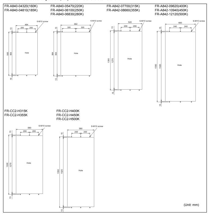
• Shift and removal of a rear side installation frame For the FR-A840-04320(160K) to FR-A840-06830(280K)
