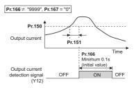
Zero current detection (Y13 signal, Pr.152, Pr.153, Pr.167) If the output during inverter running remains lower than the Pr.152 setting for the time set in Pr.153 or longer, the zero current detection (Y13) signal is output from the inverter's open collector or relay output terminal.
