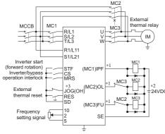
Electronic bypass sequence connection diagram
