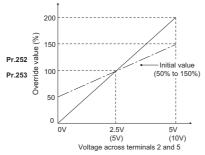
When Pr.868 (Pr.858) = "4", the terminal 1 (terminal 4) values are set to the stall prevention operation level.
