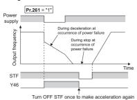
Continuous operation function at instantaneous power failure (Pr.261 = "2, 12, 22")
