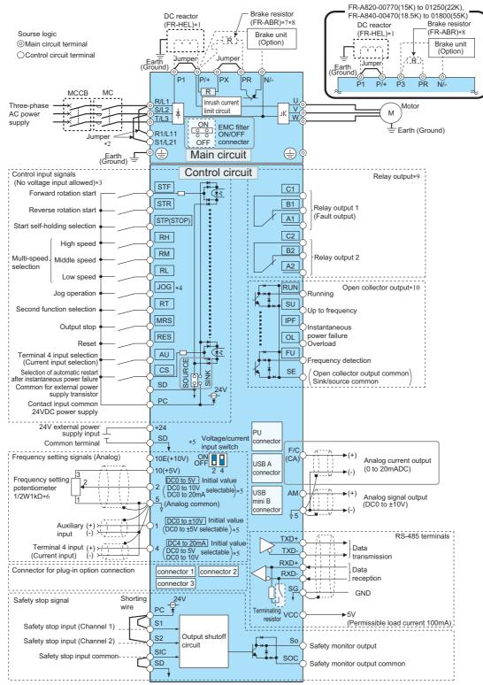
For the FR-A820-03800(75K) or higher, the FR-A840-02160(75K) or higher, and when a 75 kW or higher motor is used, always connect a DC reactor (FR-HEL), which is available as an option. (To select a DC reactor, refer to page 22, page 171, and select one according to the applicable motor capacity.)
