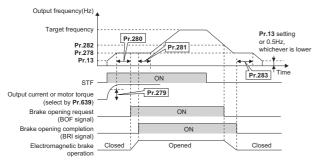
When Pr.292 = "8" (without brake opening completion signal input)
