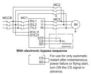
Only with restart after instantaneous power failure
